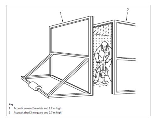
Table B.4 Measured sound reduction given by types of partial enclosure
